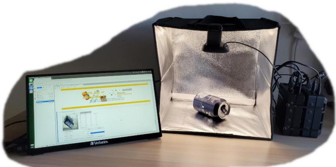
The Project Equipment, a portable monitor and two combined Seeed reComputer J1010 units hosting the NVIDIA Jetson Nano Jetpak project code
