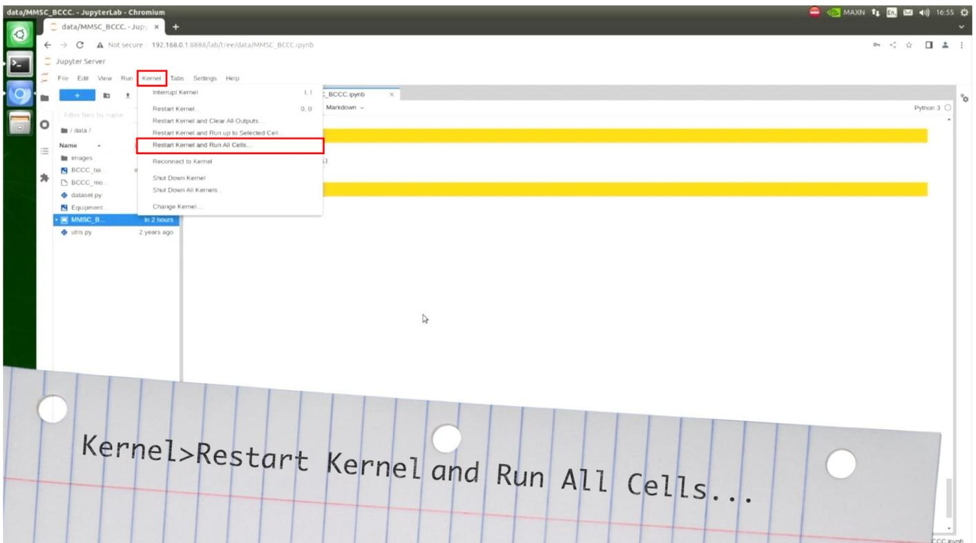
To get the system up and running and be able to operate the identification, go to **Kernel>Restart Kernel and Run All Cells...** and click on **Restart** when it appears.
