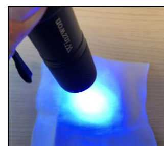
Step 3 - Turn on the UV torch shine it on the sheet of material for 5 seconds
